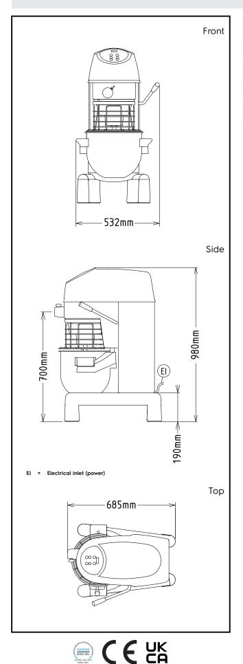
Electric Supply voltage: 200-240 V/1N ph/50/60 Hz Electrical power max.: 1.01 kW Capacity:
